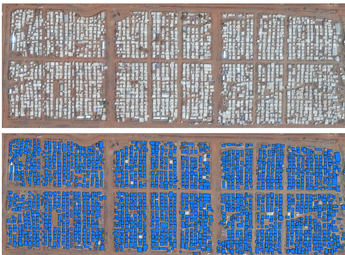
Figure 6.2: Conditioned Mask R-CNN predictions on camp Juba. Shelter diversity is low, but shelter density is high. The network can identify well shelters in this environment, but sometimes fuses neighboring shelters together.
