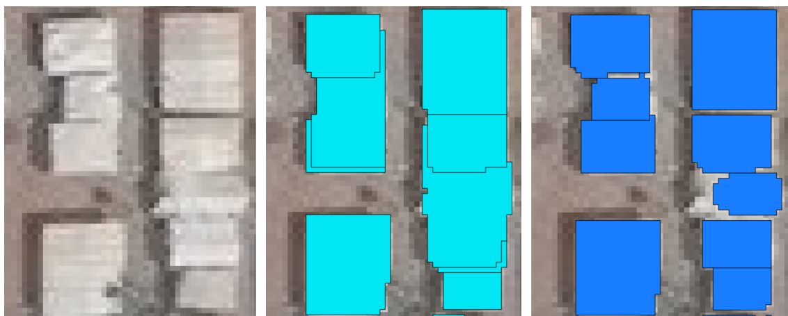
Figure 6.5: Effect of Network conditioning. From left to right, camp image, mask R-CNN without conditioning, mask R-CNN with conditioning. Indeed, the second network identifies better the boundary between the shelters, although the first one already approximately covers the total shelter area.
